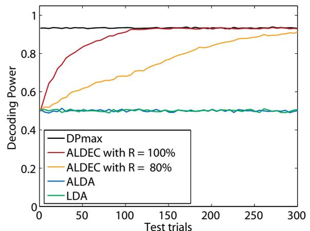
Fig. 2. **Decoding power over time for  $90^\circ$  rotation between training and feedback** LDA and ALDA show a decoding power at chance level 0.5. If an error signal with reliability of 100% or 80% is additionally considered, the decoding power nearly reaches DP max after 150 or 300 trials, respectively.
