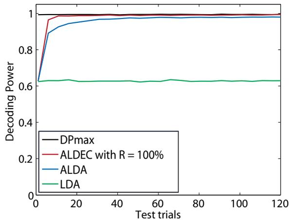
Fig. 3. **Decoding power over time for a linear shift between training and feedback.** The class distributions with distance 5 and covariance  $\begin{pmatrix} 1 & 0 \\ 0 & 1 \end{pmatrix}$  were linearly shifted by 10 and rotated by  $20^\circ$  from training to feedback session. In this case, the performance of ALDA comes very close to the one of ALDEC 100%, and to the maximal decoding power. LDA is not able to track the changes and its decoding power stays at chance level 0.5.
