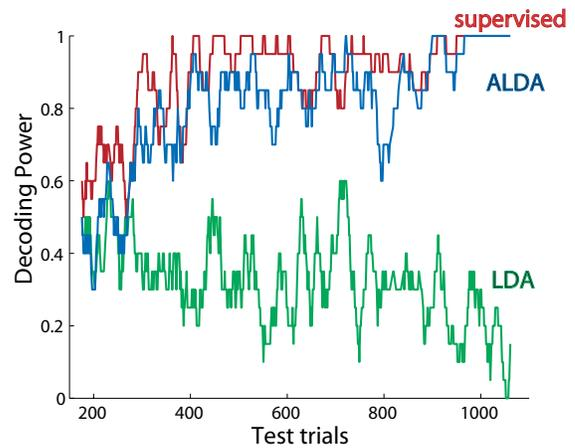
Fig. 4. **Adaptive vs. non-adaptive LDA for EEG-BCI data** In a binary task of the BCI-Competition III, data set IIIb, ALDA achieves much higher decoding power as the static LDA, nearly as high as for the supervised case.
